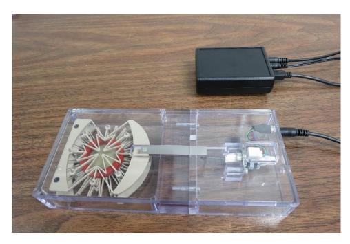
10. Place unit in incubator and begin test by using the push-button switch on the front of the control unit. A single push will start and stop the test sequence. A double push will cause the actuator to advance to the load position before pausing the sequence. A push and hold for 5 seconds will advance the actuator and reset the test sequence to the beginning.
