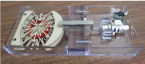
8. Fill test chamber with media OR fill test region inside containment ring with media
