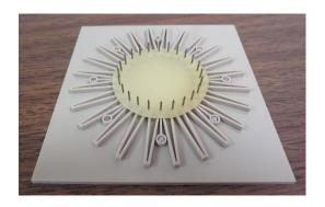
3. OPTIONAL: Place flexible containment ring on top of pins and press to mount. It may be necessary to use a silicone paste to ensure a good seal between the containment ring and the substrate.
