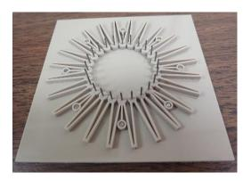
2. Place membrane on top of puncture pins and press to mount specimen
