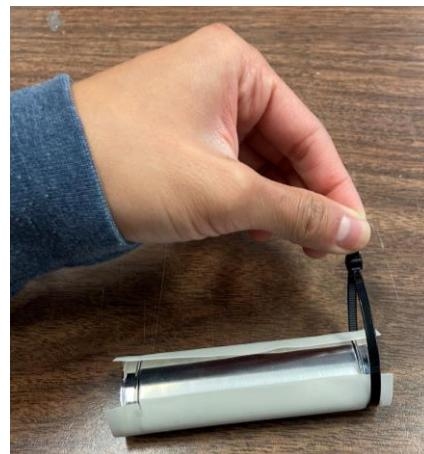
3. Use the zip tie tool to ensure the zip ties are pulled taught to secure the membrane material to the loading rings. Cut the excess on the zip ties.
