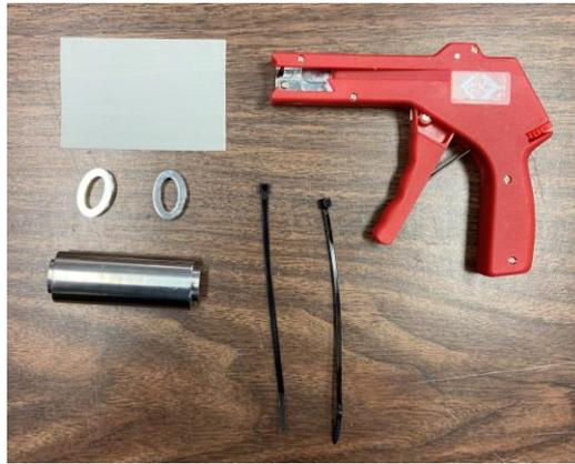
2. Slide the loading rings around the mounting bar and mount the membrane material to the loading rings with zip ties.
