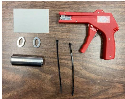
2. Slide the loading rings around the mounting bar and mount the membrane material to the loading rings with zip ties.
