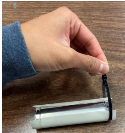
3. Use the zip tie tool to ensure the zip ties are pulled taut to secure the membrane material to the loading rings. Cut the excess on the zip ties.
