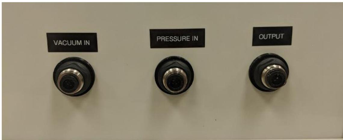
For these systems, please ensure to connect both these inputs to their respective supplies even if only one will be used in your test sequence. This is required to completely seal the system to allow fine control of the internal pressure.
