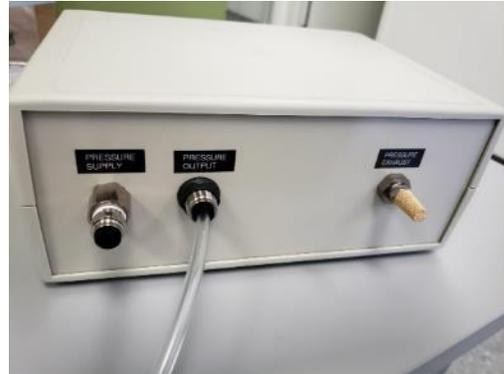
2. Connect a pressurized air supply to the control box via the pressure supply port. This could be a 1/4-inch air compressor quick-connect coupler (*Option 1*) or a push to connect fitting for 1/4 inch tubing (*Option 2*) (supplied but not installed), depending on your pressurized air supply.
