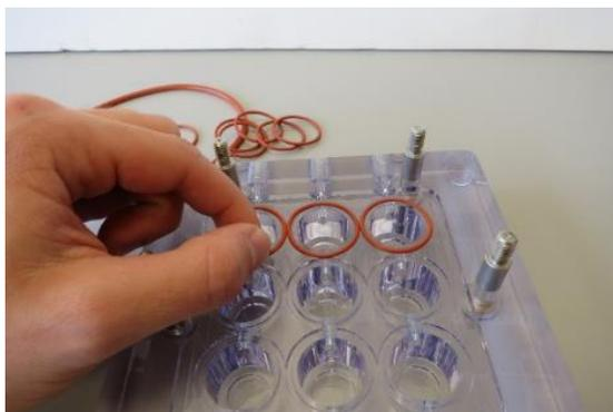
5. Collect the small and large O-rings from the grooves in the specimen holder.
