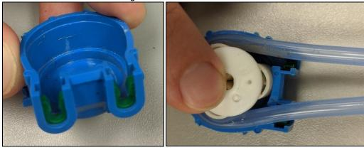
6. Slide the tube into each of the green clips and place the back cap back on and snap the pump head back in place with the new tube.
