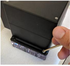
1. Begin by removing the M5 and M6 fasteners and lifting the control unit off the well plate.
