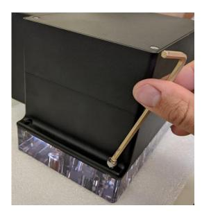
5. Next, place the control unit on top and fasten it to the well plate using the M5 and M6 fasteners. The diagram below shows a top view of how the wells are numbered.
