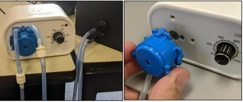
3. Once the pump head is removed take the back cover off to expose the rotating cam and tubing. With the back cover off lift the tubing up and out of the green clips which are used to hold it in place. Once the green clips are removed you can lift the cam and tubing out of the assembly. Be careful as the cam is made of loose parts that can roll away.
