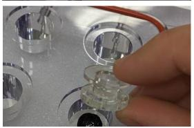
3. Insert your specimen spacer that corresponds to your sample size into each of the 6 wells, place sample, and then place the hourglass shaped plunger on top. Ensure that they are flush with the top of the well plate. If not, additional spacers or a larger specimen may be required.
