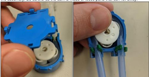
4. With the cam and old tube removed, you can remove the luer lock barbed fittings and place them into the new tube.
