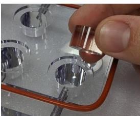
Remove the membrane and sterilize the spacers and membrane or well plate if needed. Next insert the spacers provided for your specimens.
