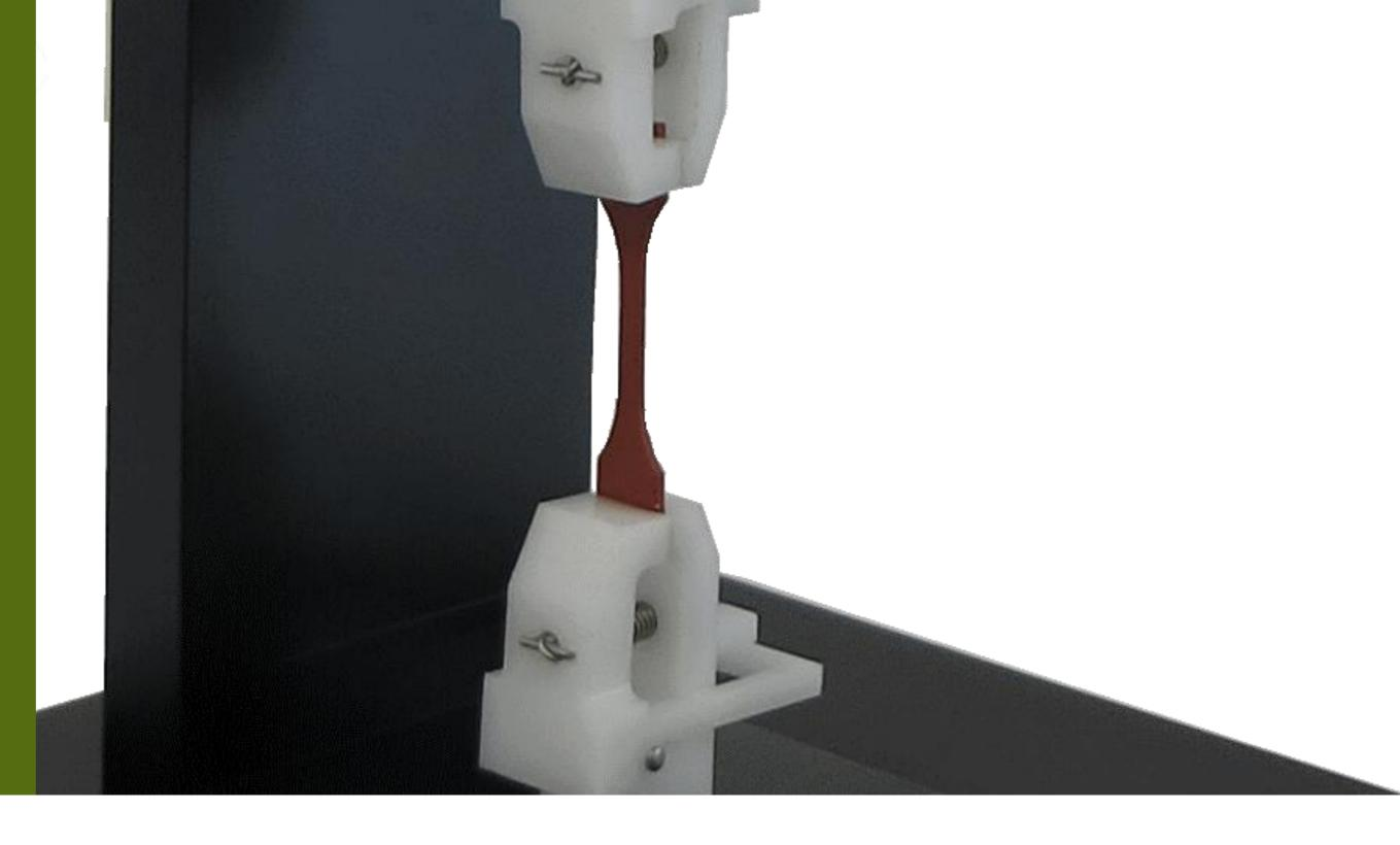
The UniVert software enables users total control over the test protocol. Real-time graphing and test monitoring provides feedback during the test while the resulting force and displacement data are stored for further analysis.
