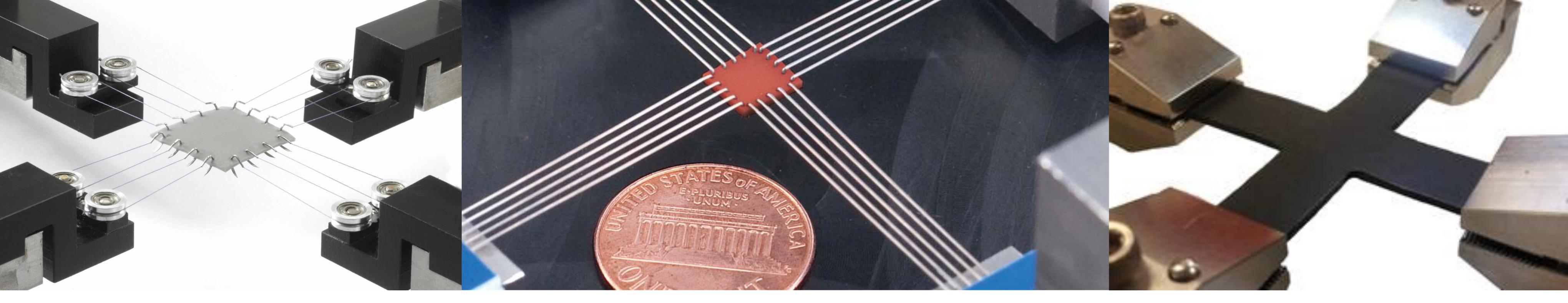
A variety of gripping methods are available for the BioTester. The patented BioRakes allow for fast and accurate mounting of specimens as small as 3mm. A tether mounting system allows for uniform force at each attachment point. Grips are useful for cruciform specimens and uniaxial tests.
