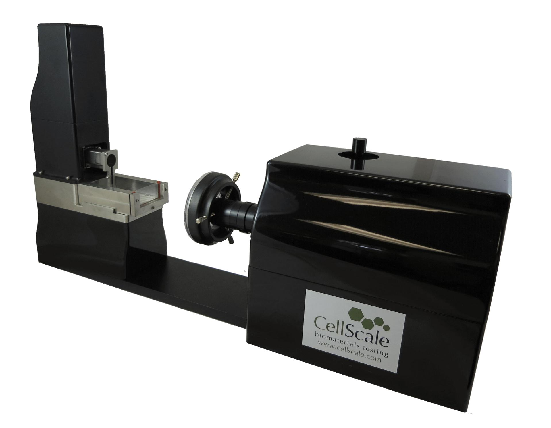
and compression testing at low forces. This report outlines the results of compression testing of a soft gel material using 3 methods: cylindrical specimen compression of cylindrical specimens, compression of spherical specimens, and indentation testing using a spherical indentor. The results show that all three techniques are viable for measuring the stiffness of gel materials.
