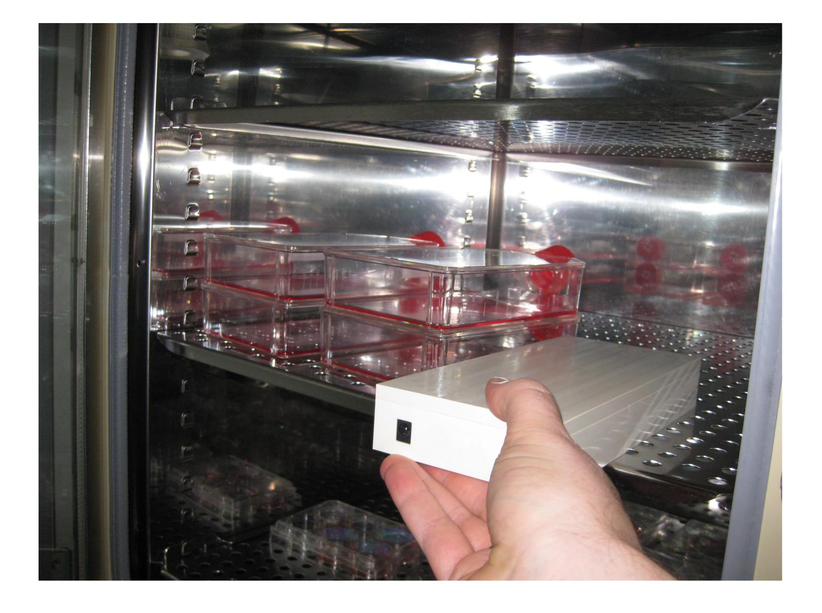
All components in contact with the culture can be autoclaved and the device can be run inside an incubator environment.
