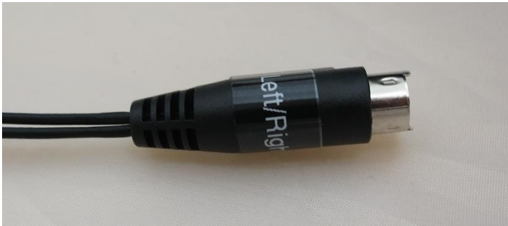
The piezo stage connectors are labelled according to the port they should be plugged into
