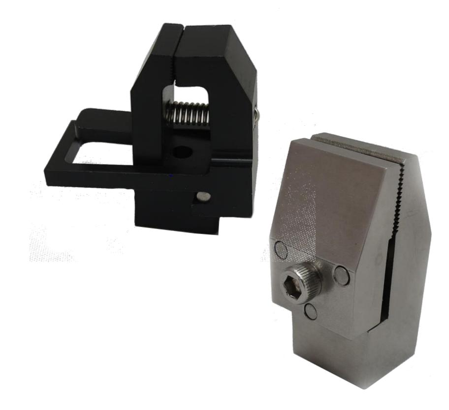
Soft materials are easily damaged by over-clamping, but it is also important to have sufficient clamping force to prevent slippage. Using spring-closure clamps ensures a consistent force with every test.
