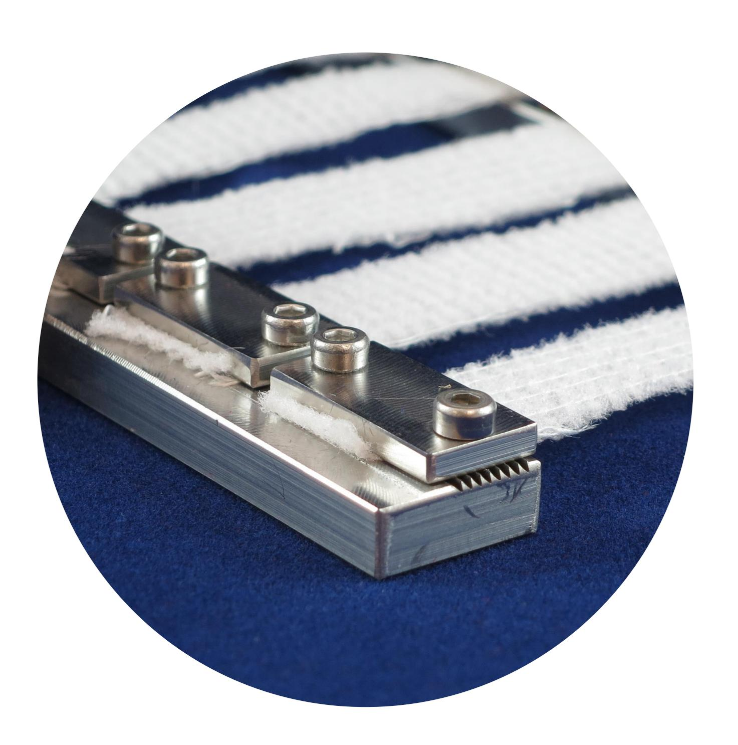
Stainless steel grips secure the specimens at each end. The spacing and geometry of these grips can be customized to suit a variety of specimen sizes and materials
