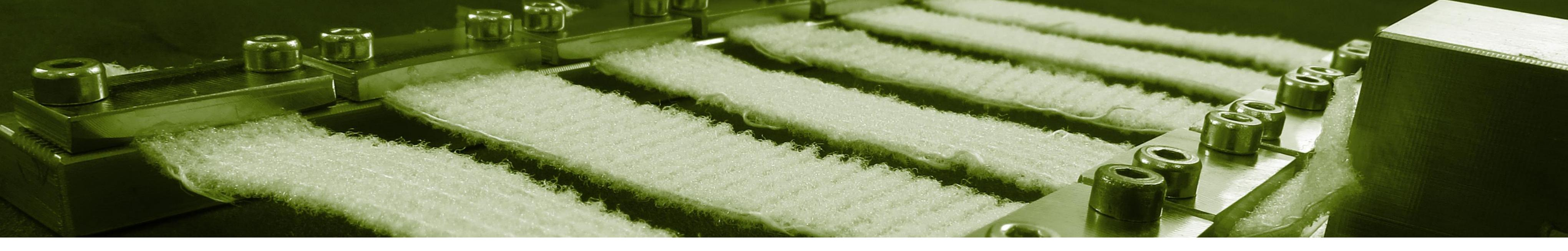
The MechanoCulture T6 can be programmed to run constant velocity or sinusoidal stretch patterns. Magnitudes, frequencies, rest periods, and cycle counts can all be specified in the software application and programmed to the device.
