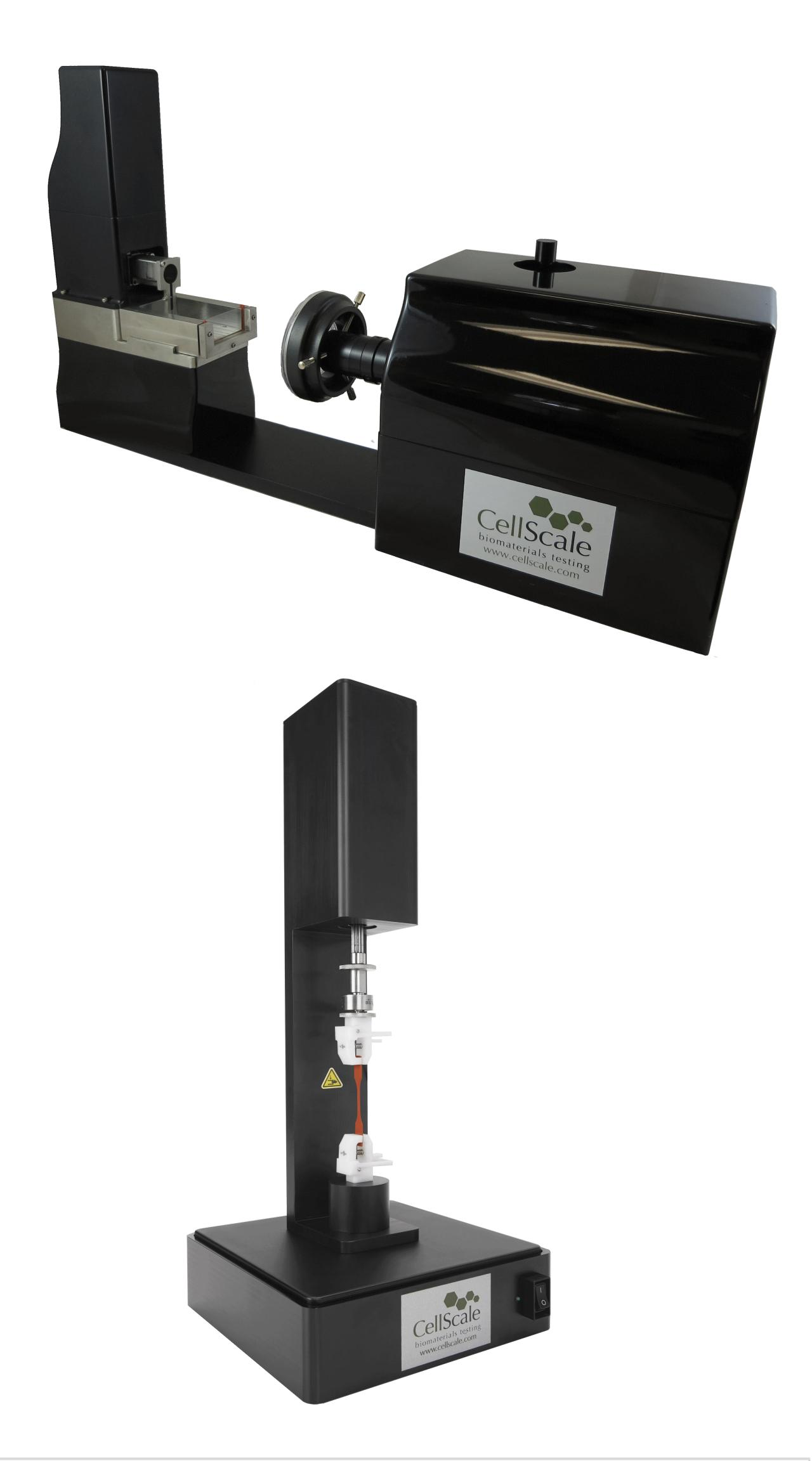
This report outlines the results of tension testing of an elastic filament using 2 methods: mechanical grips and a conventional load cell (UniVert) and 3-point tension testing with a high-resolution force transducer and high-magnification imaging (MicroTester). The 3-point technique varies from the conventional in-line technique in that the force sensor does not need to be fixed to the specimen. This difference simplifies the test setup for small, delicate samples.
