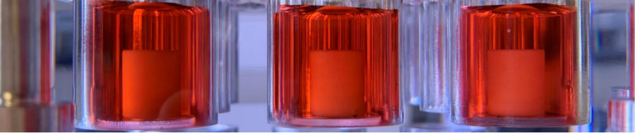
The MechanoCulture TR can be programmed to run constant velocity or sinusoidal compression patterns. Magnitudes, frequencies, rest periods, and cycle counts can all be specified in the software application and programmed to the device.
