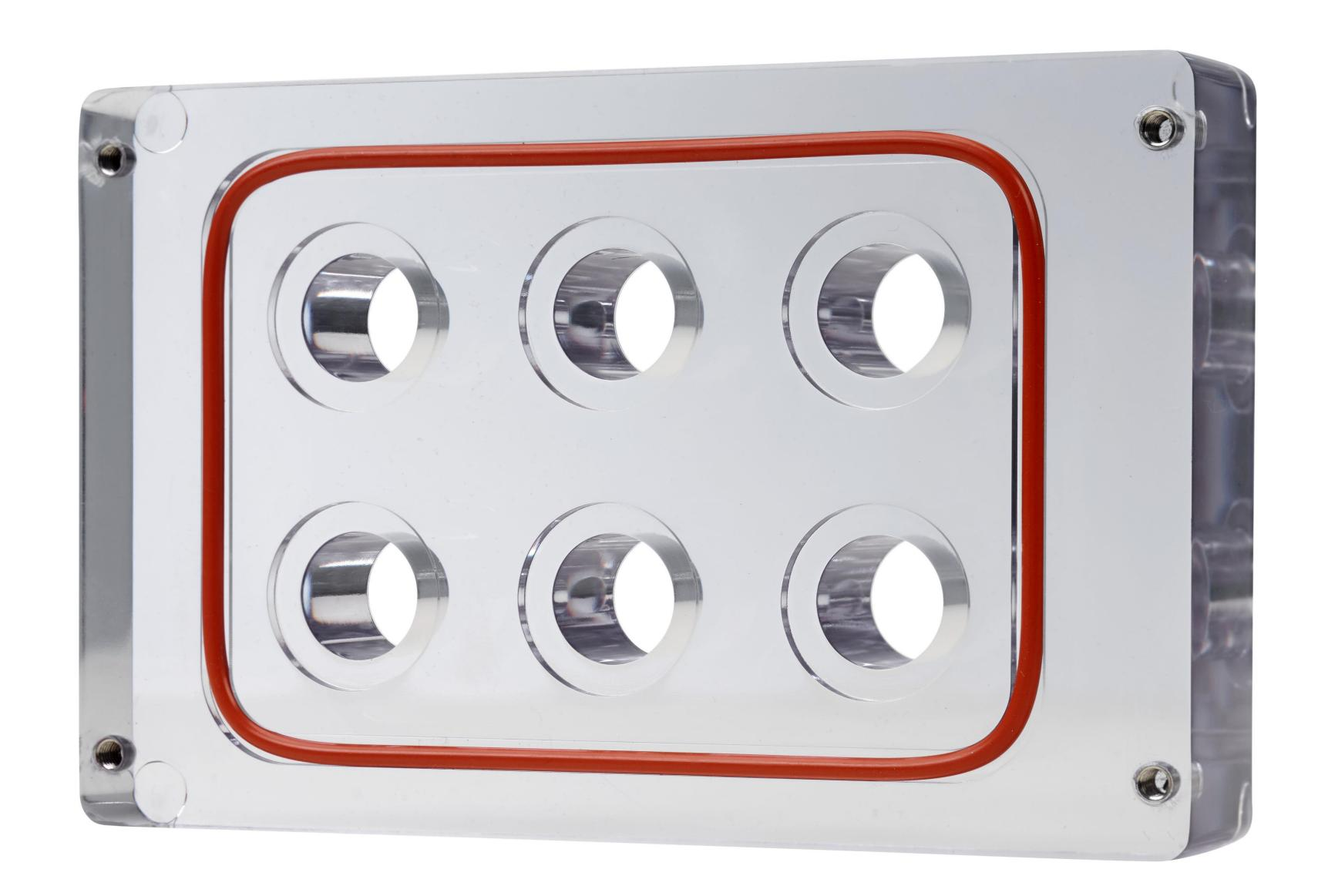
All components in contact with the culture can be autoclaved and the device can be operated inside an incubator environment.
